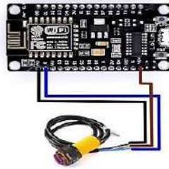
Fig 2 Connecting the motion detection sensor to the Arduino board
